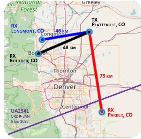
Fig. 2. Map of the Zephyr Meteor Radar Network showing transmit and receive locations and the flight path of the aircraft signature seen in Fig. 1
