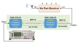
Fig. 1. Block diagram of the proposed LO chain module used for six-port receivers.
