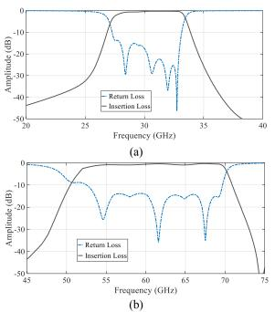
Fig. 2. The simulation S-parameters of (a) the first BPF (BW: 28 to 33 GHz), (b) the second BPF (BW: 56 to 66 GHz).
