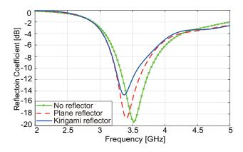
Fig. 2. Reflection coefficients of the antennas shown in Fig. 1 (a)-(c).
