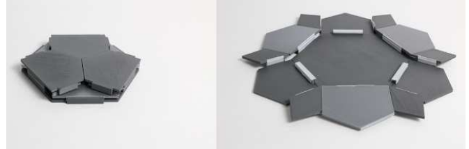
Fig. 3 The hexagonal RA structure at its stowed (left) and deployed (right) states.
