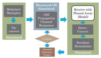
Fig. 1. Flow chart of the evaluator simulation.
