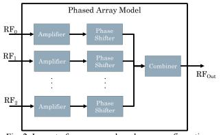
Fig. 2. Layout of a common phased array configuration.
