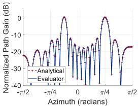
Fig. 3. Spatial responses of an analytical beamforming solution and the evaluator with ideal hardware models for known incident angles.
