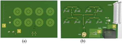
Figure: (a) Proposed 2x4 dual mode microstrip phased array antenna aperture and (b) Beamforming network layer with RFICs.
