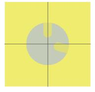
Figure 1: Asymmetric ENNZ-MTM-lined Aperture
