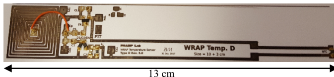
Fig. 1 Photograph of an IJP WRAP temperature sensor on paper substrate.
