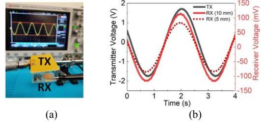
Fig. 5. (a) Test set-up at 10 mm, (b) Measured TX and RX voltages.
