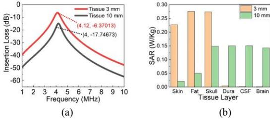
Fig. 4. (a) Insertion Loss  $S(2,1)$  and (b) SAR at different tissue depths.
