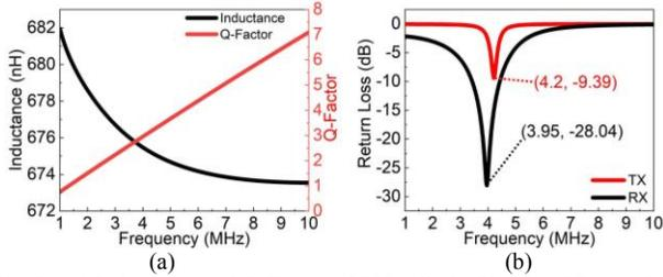
Fig. 3. (a) Inductance and Q-Factor of RX coil, (b) Simulated Return loss ( $S_{11}$ ) of the TX and RX modules.
