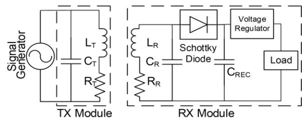
Fig. 1. Block diagram of a WPT System.
