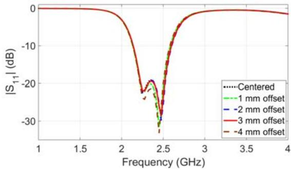
Fig. 2.  $|S_{11}|$  versus frequency for different offset distances.
