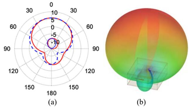
Fig. 5. (a) 2D gain patterns of the antenna in principal planes [ $\phi = 0^\circ$  co-pol (red-solid),  $\phi = 0^\circ$  x-pol (red-dotted),  $\phi = 90^\circ$  co-pol (blue-dashed),  $\phi = 90^\circ$  x-pol (blue-dotted), ]. (b) 3D pattern of the antenna.
