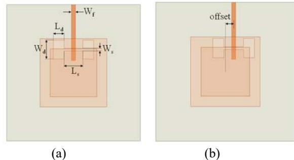
Fig. 1. (a) Geometrical parameters of the aperture and feed line. (b) The offset configuration of the aperture.
