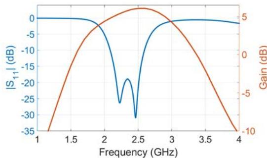
Fig. 4.  $|S_{11}|$  and gain versus frequency for the dual-polarized aperture coupled patch antenna.
