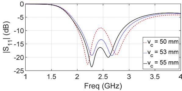
Fig. 3.  $|S_{11}|$  versus frequency for different values of  $v_c$ .
