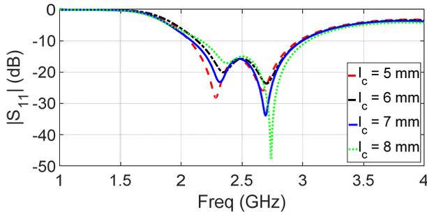
Fig. 5.  $|S_{11}|$  versus frequency for different values of  $l_c$ .
