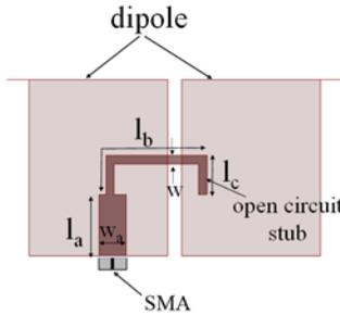
Fig. 4. The balun and design parameters.
