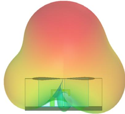
Fig. 2. 3D pattern of the dipole antenna at 2.45 GHz.
