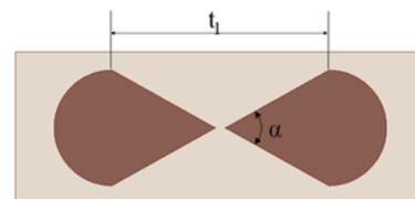
Fig. 2. Top view of the conical bowtie dipole antenna.
