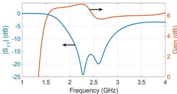
Fig. 6.  $|S_{11}|$  and gain versus frequency for the optimized printed conical bowtie dipole antenna.
