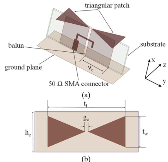
Fig. 1. The bowtie dipole antenna. (a) 3D, (b) top view.
