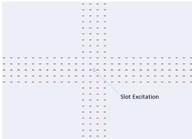
Fig. 2. The cross-shaped 2D periodic leaky-wave antenna fed by a slot in the ground plane.
