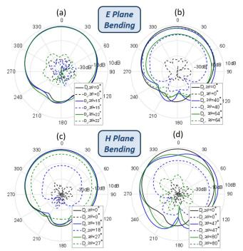
Fig. 4. Radiation pattern variations with respect to bending angles for E plane bending in (a) and (b), and H plane bending in (c) and (d).
