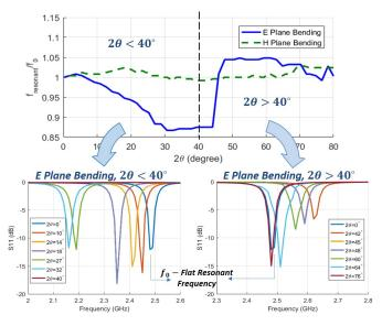
Fig. 2. Frequency variations of the bending effects on both E and H plane. The normalized frequency shift is plotted with respect to bending angles for the rectangular patch antennas. The E plane frequency shift due to bending splits into two regions, with left shift on slightly bent region  $(2\theta < 40^{\circ})$ , and right shift on severely bent region  $(2\theta > 40^{\circ})$ .
