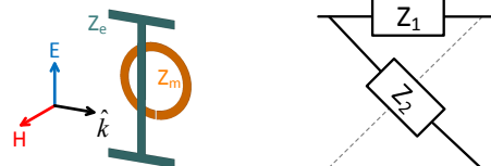
Fig. 1. A Huygens' unit cell and the equivalent lattice network.
