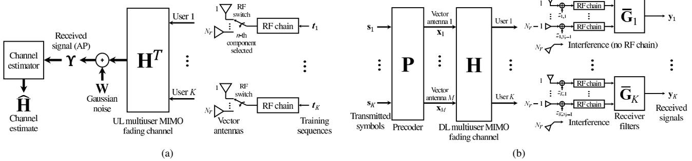
Fig. 1. (a) Uplink and (b) downlink system models for polarimetric interference alignment.
