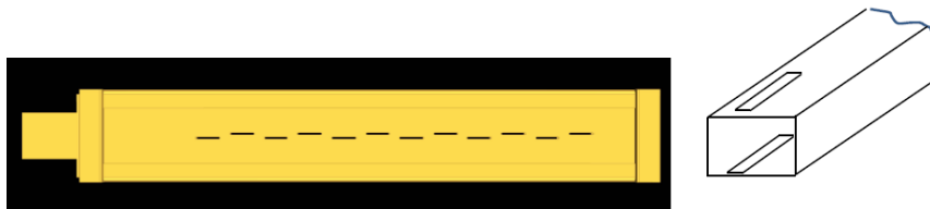
Figure 1 Linear array of slot pairs for omnidirectional pattern
