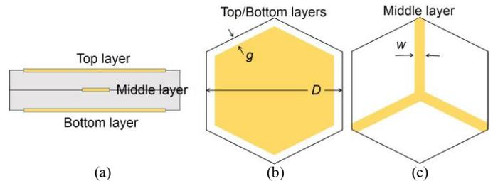
Fig. 1. Proposed FSS unit cell, (a) top and bottom layers, and (b) middle layer.
