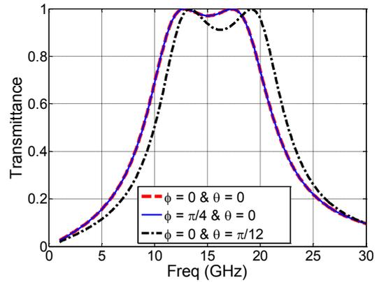
Fig. 3. Effect of incident angle and polarization on FSS response.
