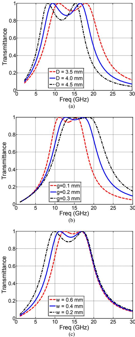
Fig. 2. Parametric study results of transmittance response, (a) unit cell size with a fixed  $g$  and  $w$  values, (b) inductive loading width with fixed unit cell and capacitive patch size, and (c) capacitive patch loading with fixed unit cell and inductive loading width.
