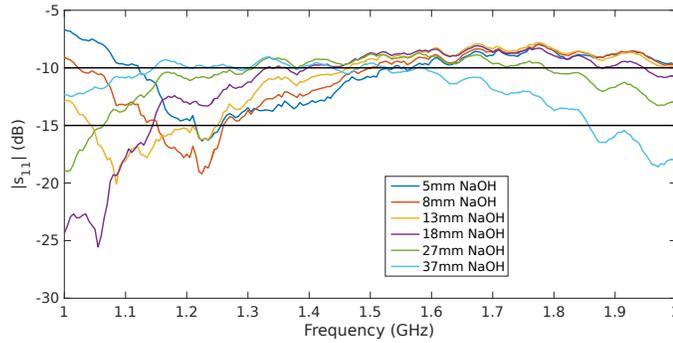
Fig. 3. Bottom fed with stub: EGAIn length of 41mm
