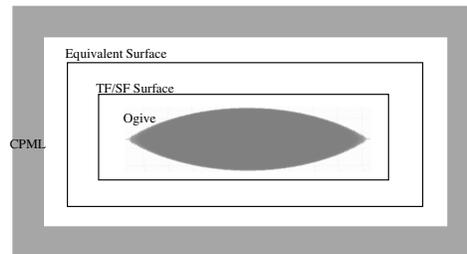
Figure 1: A 2D view of the ogive surrounded by TFSF, near to far-field transformation surface and outer absorbing boundary conditions.
