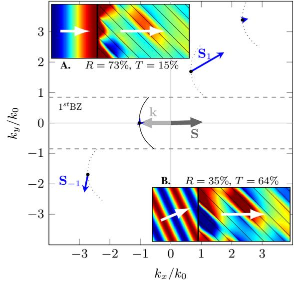
Fig. 2. The  $k$ -space map for propagation through the MDMDM structure at an angle of  $45^\circ$  to the layers. The interface was also oriented at  $45^\circ$  so this mode could be excited by a normally incident plane wave (inset A). The EFCs correspond to modes consistent with this interface. Inset B shows the fields given a single oblique plane-wave excitation of the same normal mode.
