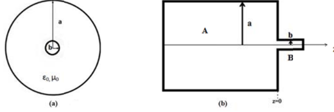
Figure 1 Empty cavity with exit hole geometry [(a) transverse plane (b) side view]
