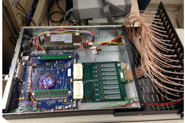
Fig. 1. The FPGA development board known as ROACH (blue PCB) was used to process PAF data after digitization by the x64 ADC board (green PCB).
