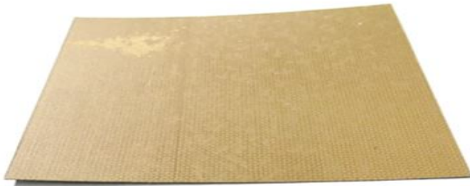
Fig. 2. Carbon epoxy layup layered with phosphor bronze mesh
