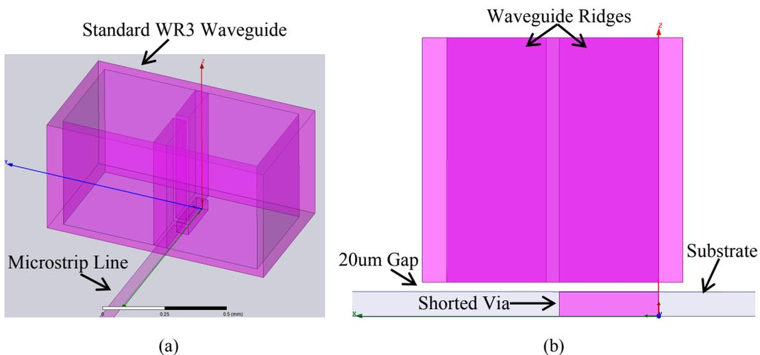
Figure 1. Transition from the standard WR3 waveguide to the microstrip ports of a given device; (a) 3D view and (b) side view.
