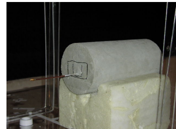
Figure 1: Antenna embedded in concrete cylinder.
