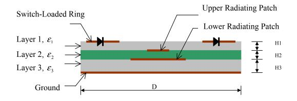
Figure 1: Cross Section of a Reconfigurable Dual Band Microstrip Antenna
